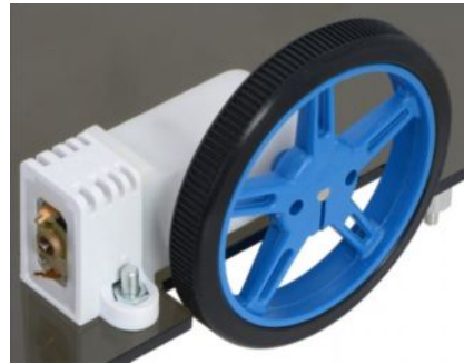
Fixing of the motor and driving wheel
