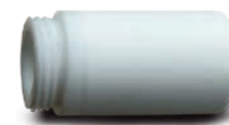
F5300 - Teflon (PTFE) sensor cover (white colour), with increased resistance against splashing water, non-absorbent surface, does not rust. Porous size 25µm. Temperature range -40°C to +125°C.
